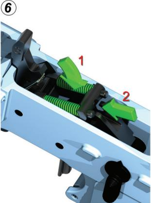
Reverse the steps to uninstall the parts and reinstall with a different spring combination to change trigger pull according to the table. Use a pointed tool inserted into the toggle pivot at the arrow for convenient removal and reinsertion.
