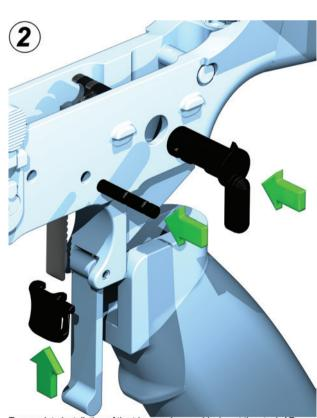
To complete installation of the trigger subassembly, insert the stock AR 0.154-inch diameter pivot pin in the usual way (just like you would install a stock AR trigger). Install the safety-selector and grip. Install trigger shoe during trigger insertion, or after, as shown.
