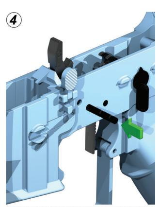
Complete installation of the hammer subassembly by inserting the stock AR 0.154-inch diameter pivot pin like you'd install a stock AR hammer.
