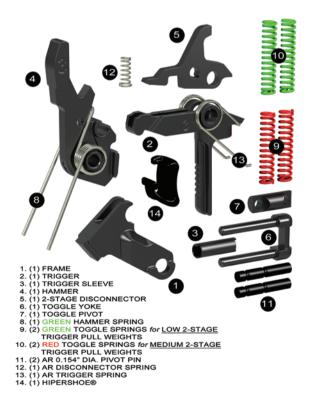
The X2S™ MOD-3 fire-control group (FCG) parts are shown in the figure by name and quantity. The trigger portion comes preassembled TRIGGER SLEEVE, etc. It "drops" in complete; just pin in-place.
