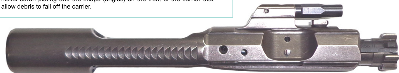
Below: The LWRC International Enhanced Bolt Carrier group. The carrier key is screwed and then pinned into the bolt carrier. There is no bolt carrier key, no screws to break and no separate key to have gas leakage. Note the nickel-boron plating and the shape (angles) on the front of the carrier that allow debris to fall off the carrier.
