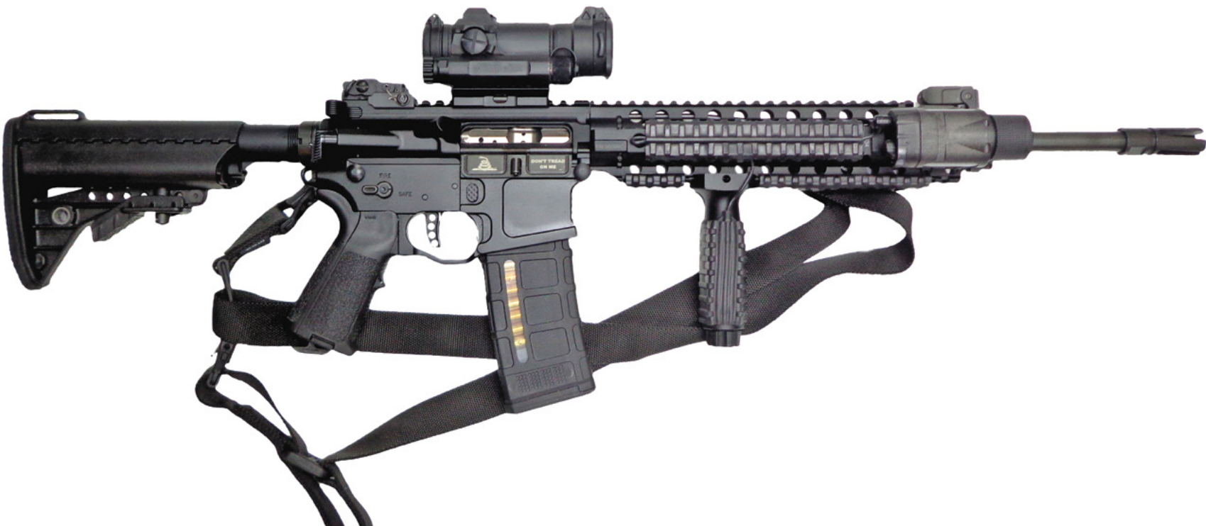
Above: The first rifle to be examined is based on the Mega Arms matched receivers. Notice the Magpul Gen 3 PMag with Maglevel as well as the Aimpoint Comp4S. Below: The receiver extension end plate is manufactured by Full Circle Warrior and called the Close Quarter Defense. You can also see the Yankee Hill Machine EZ Pull rear takedown pin and the Iron Viper checkered pattern forward bolt assist.
