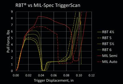
Note the reduced pull weight and reduced creep of RBT compared to typical OEM MIL\_spec triggers. No other trigger delivers this performance at OEM wholesale pricing. The pull energy is plotted below and is the calculated area under each scan plot.
