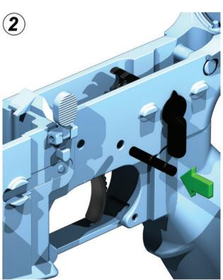
To complete installation of the trigger subassembly, insert the stock AR 0.154-inch diameter pivot pin in the usual way (just like you would install a stock AR trigger).
