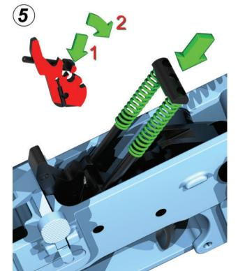
Inspect the fire-control for proper toggle spring installation and function whenever live-fire exercise is intended, especially if you had the fire-control installed by someone else, or if you loaned your rifle to someone else.
