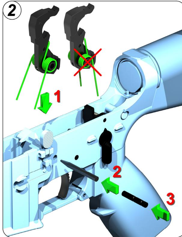
Choose the red spring for a 5½+ lb. trigger pull weight or the silver spring for 4½+ lbs. Install the hammer sub- assembly into the lower receiver just like you would a stock AR hammer, making sure the hammer spring's arms nest in the spaces on either side of the trigger in the lower receiver to retain the trigger pivot pin. Use the drift pin as desired.
