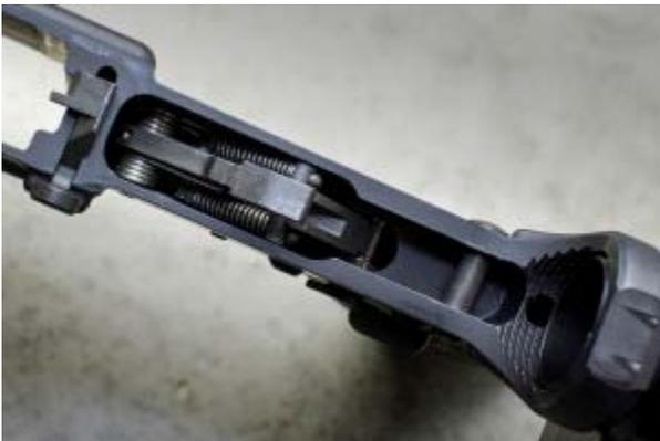
hammer’s travel the toggle springs begin to push on the hammer. This can be felt when lowering the hammer slowly by hand. Hiperfire advertises a 35% increase in hammer fall energy over the Mil-Spec design.
