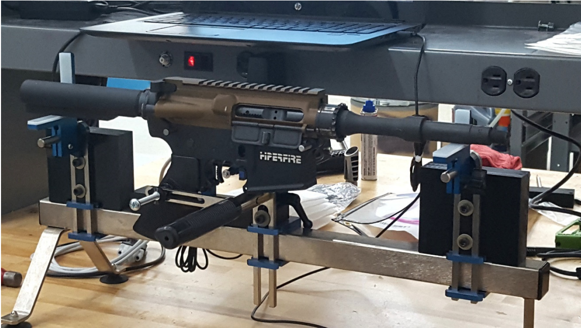
Figure 2. The TriggerScan device shown in the picture has been stiffened by blocks to stabilize the rifle holding platform to eliminate extraneous movements that could be picked up by the TriggerScan force/displacement sensor.
