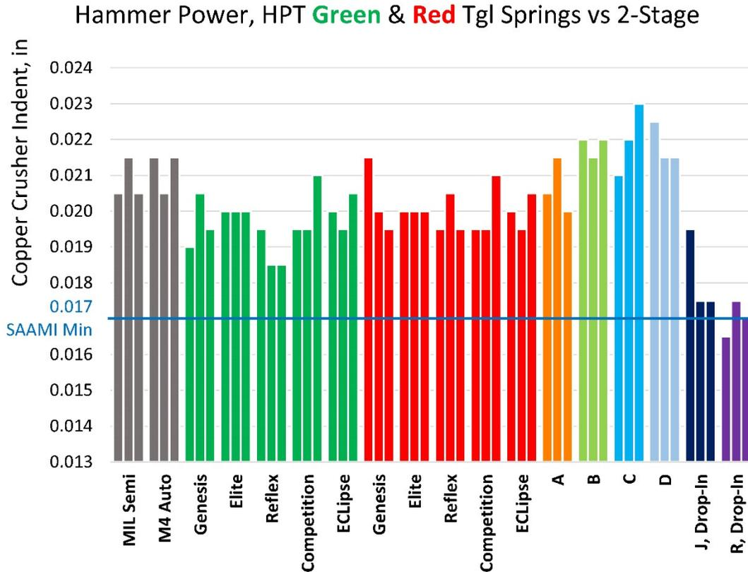
Figure 3. Copper crusher charted data is shown for HIPERFIRE HIPER-TOUCH triggers with the green and red toggle springs installed versus MIL-spec and 2-stage trigger products.
