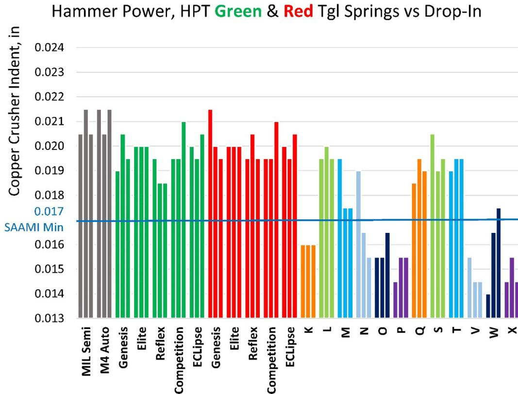
Figure 4. Compare copper crusher data for HIPERFIRE HIPERTOUCHE triggers with the green and red toggle springs installed to MIL-spec and drop-in trigger products.
