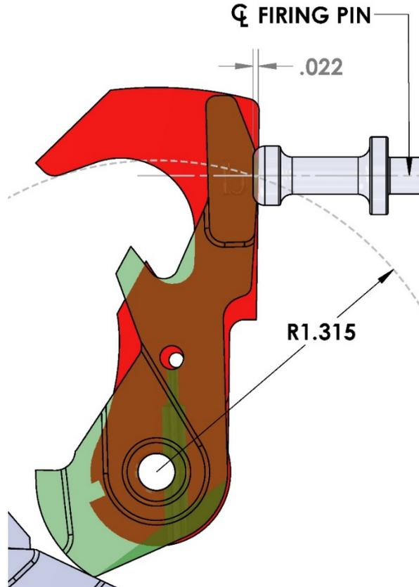
Figure 1. Compare the MIL and EDT SS hammers, where they first make contact with the firing pin and their positions when the copper crusher indent reaches a hypothetical .022" depth.
