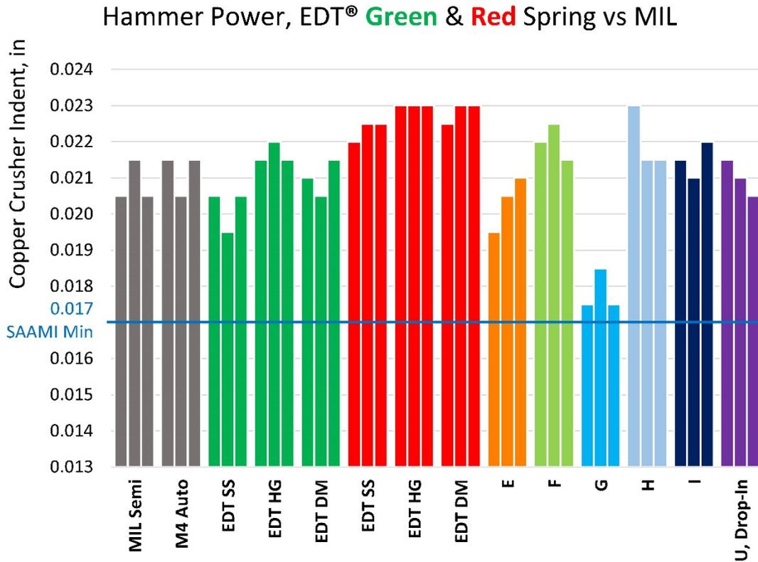
Figure 2. Compare copper crusher charted data for HIPERFIRE EDT triggers with the green and red hammer spring installed to MIL-type trigger products.
