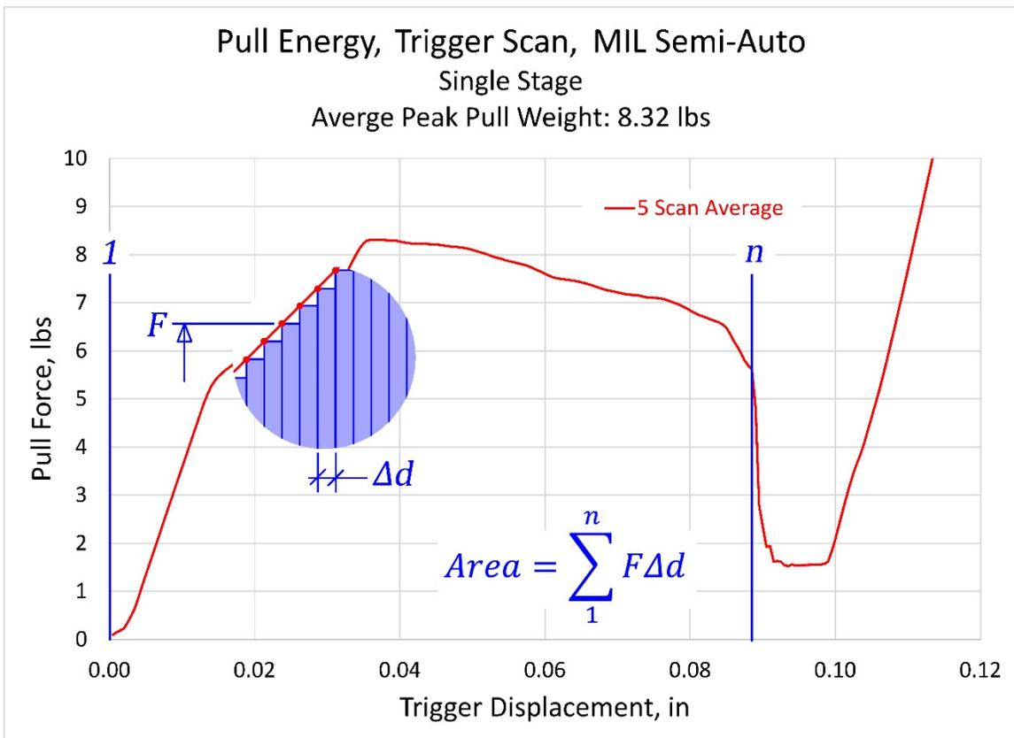
Figure 2. Summing the areas associated with each sequential pair of data points up to trigger break equals the "area under the curve."
