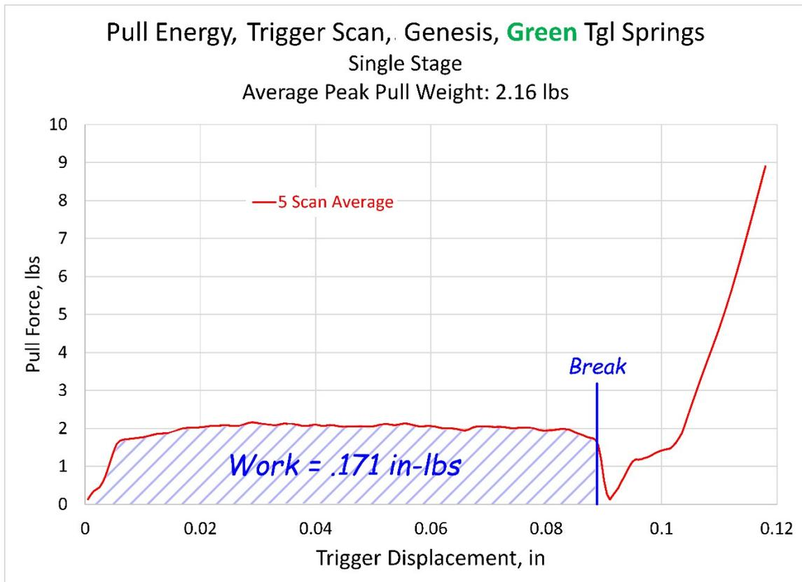
Figure 4. Chart showing the area under the curve up to trigger break, or the work or energy expended to cause trigger break and hammer release of the HIPERTOUCHE Genesis trigger with the COTE Green toggle springs installed.
