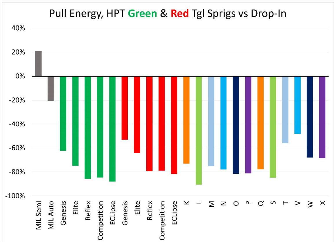
Figure 11. Chart comparing HIPERTOUCH triggers with green (green bars) and red (red bars) toggle springs to 2-stage type triggers based on pull energy to trigger break.
