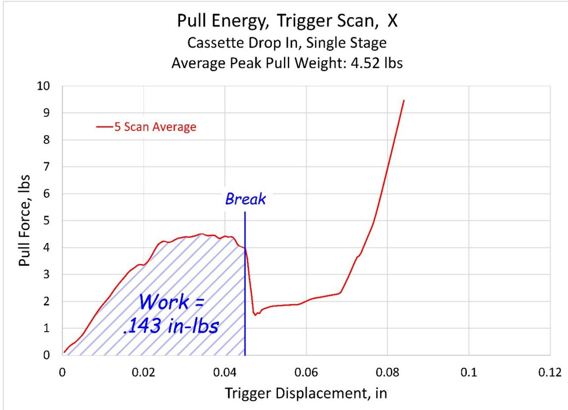
Figure 8. Chart showing the area under the curve up to trigger break for the "X" single-stage cassette drop-in trigger, or the work done (energy expended) to cause trigger break and hammer release.
