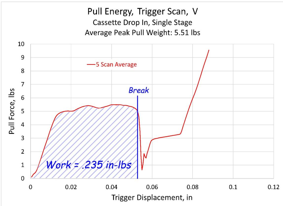
Figure 7. Chart showing the area under the curve up to trigger break for the “V” single-stage cassette drop-in trigger, or the work done (energy expended) to cause trigger break and hammer release.
