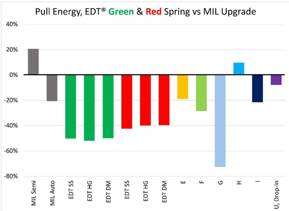
Figure 9. Chart comparing EDTs with green (green bars) and red (red bars) hammer springs to single-stage MIL type triggers based on pull energy to trigger break.
