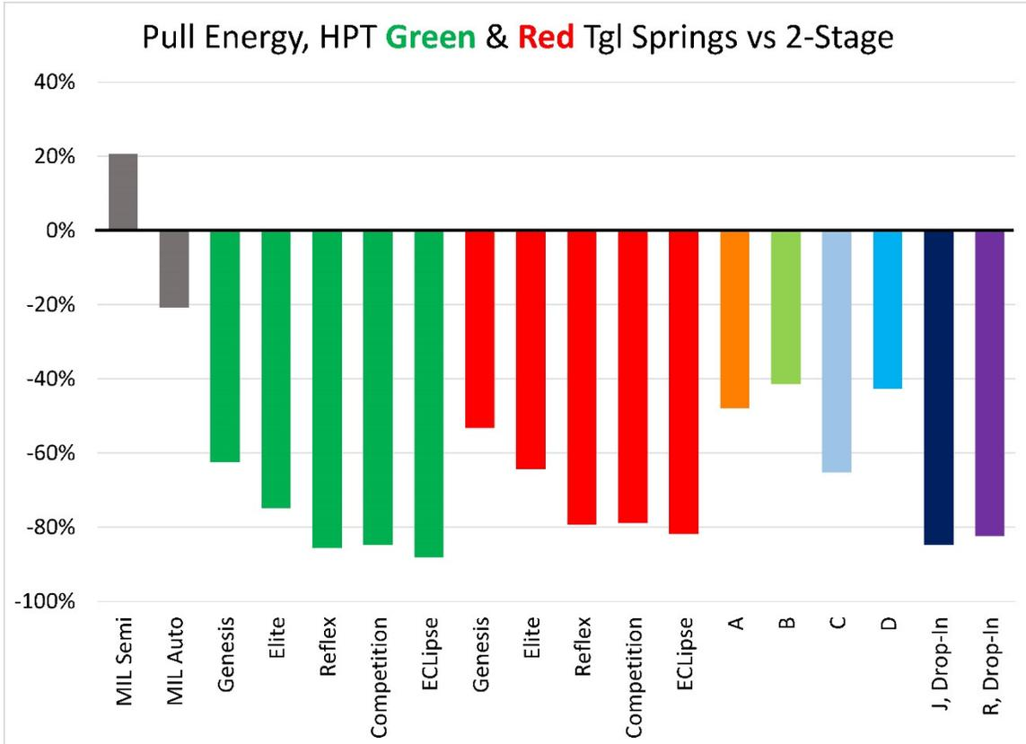
Figure 10. Chart comparing HIPERTOUCHE triggers with green (green bars) and red (red bars) toggle springs to 2-stage type triggers based on pull energy to trigger break.
