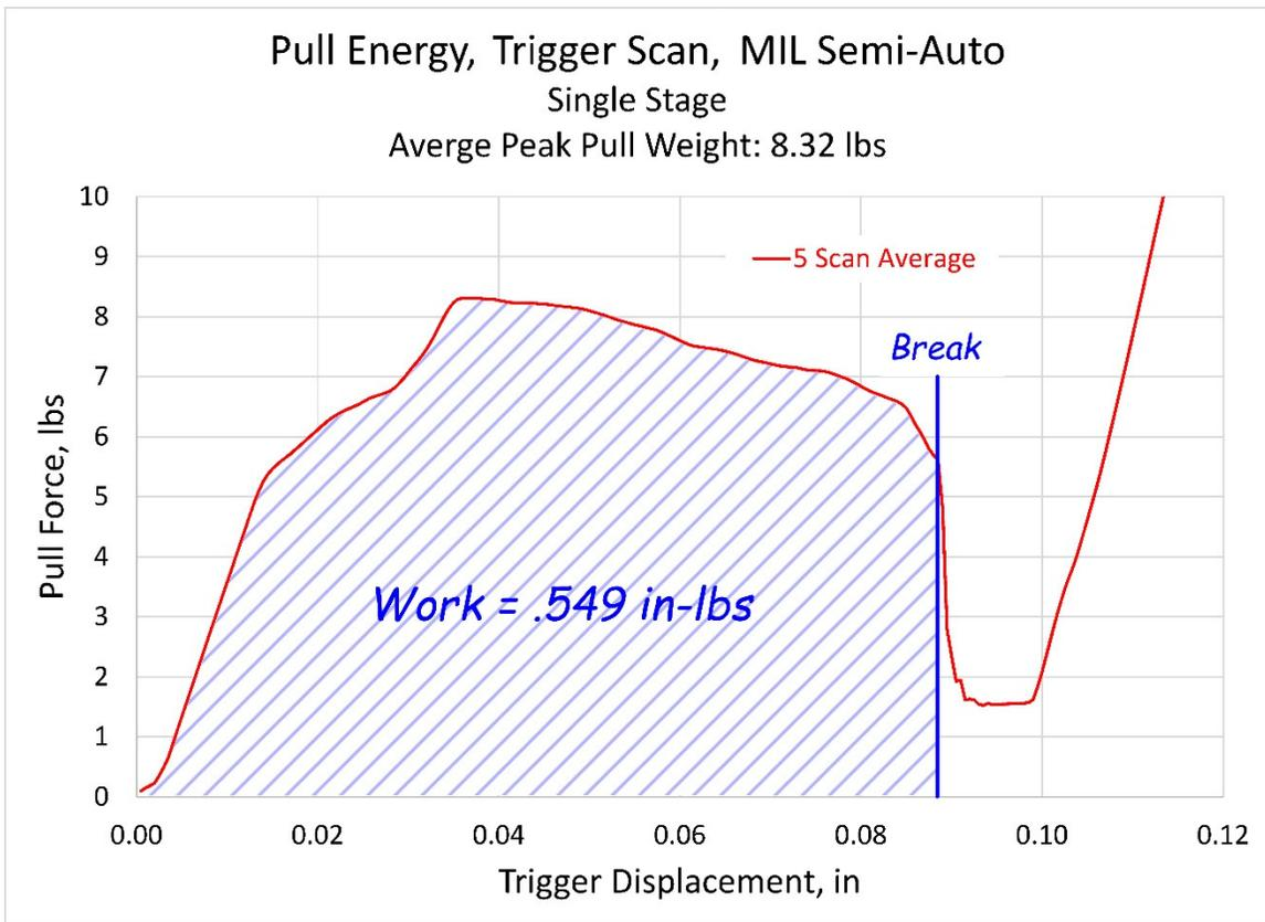
Figure 3. Chart showing the area under the curve up to trigger break, or the work that must be done (energy expended) to cause trigger break and hammer release of the MIL-spec semi-auto trigger.
