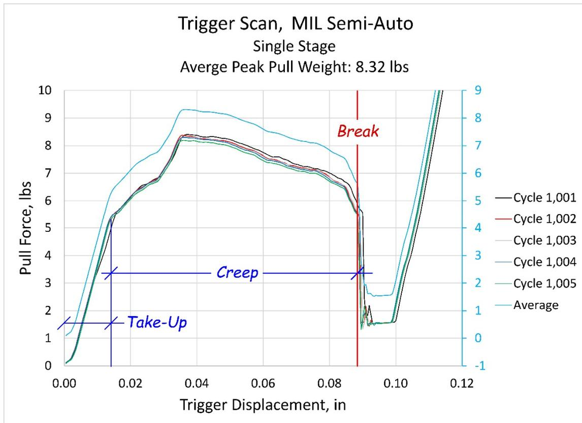
Figure 1. Chart defining wherein the trigger scan trigger break occurs — measurement data collected by TriggerScan™.
