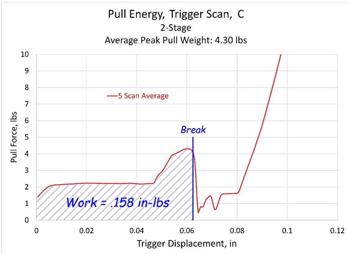
Figure 6. Chart showing the area under the curve up to trigger break for the “C” 2-stage trigger, or the work done (energy expended) to cause trigger break and hammer release.
