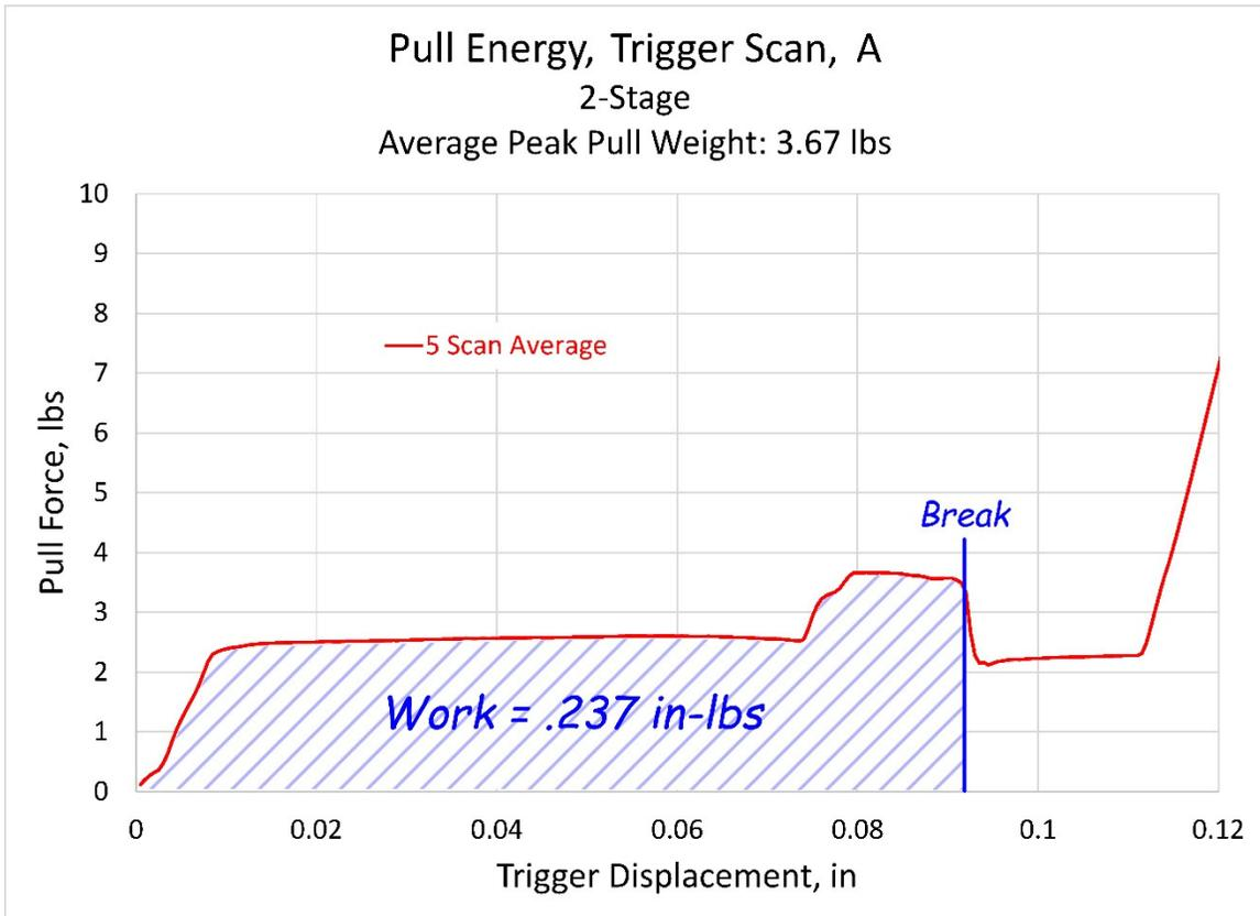
Figure 5. Chart showing the area under the curve up to trigger break for the "A" 2-stage trigger, or the work done (energy expended) to cause trigger break and hammer release.
